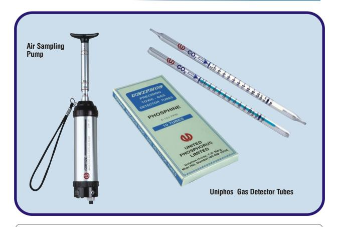
When monitoring of a toxic gas concentration is not essential but monitoring its concentration at a specific moment or at a specified interval is all that is desired, UNIPHOS short term detector tubes provide the answer.
